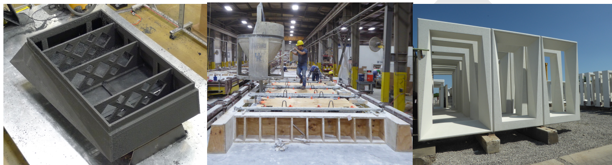
Figure 15. Additive manufacturing has been demonstrated successfully for precast concrete forms of building facades. Avenues to employ advanced manufacturing techniques, such as additive manufacturing, for energy-efficient window-to-facade integration merit additional investigation.
