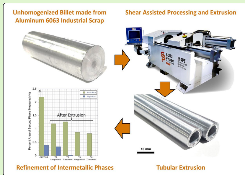
Figure 8. Illustration of using ShAPE to recycle aluminum, resulting in refined microstructure. Source: Whalen et al. 2023a.
