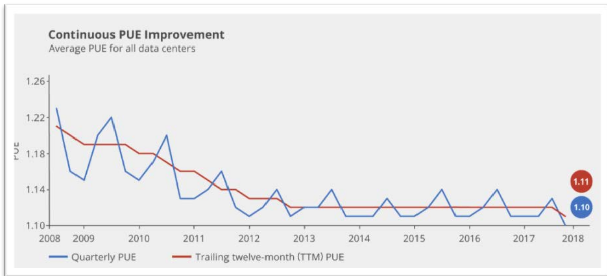
Figure 45. Power usage efficiency data for all large-scale Google data centers. Source: Google. https://www.google.com/about/datacenters/images/pue-average.png
