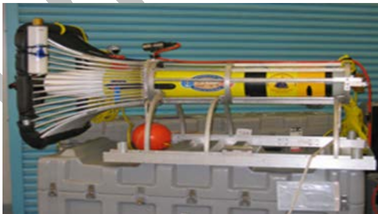
Figure 7. Underwater Remus docking station. Photo courtesy of WHOI
