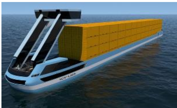
Figure 72. Port-Liner canal cargo vessel in development, capable of autonomous operation. Source: Port-Liner
