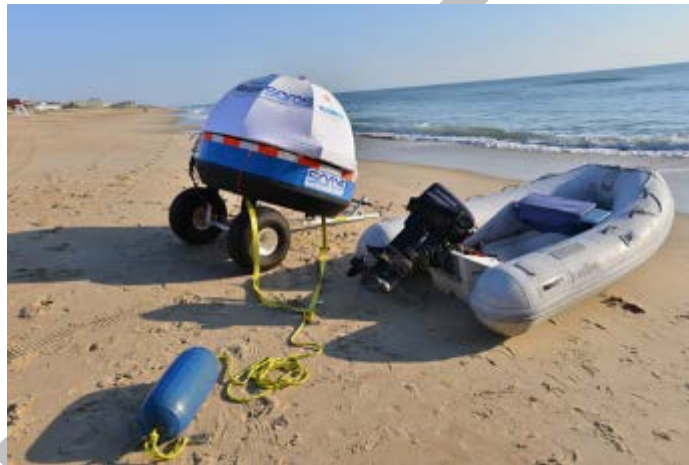
Figure 18. SAROS wave-powered desalination demonstration unit. Source: https://www.digitaltrends.com/cool-tech/saros-buoy/
