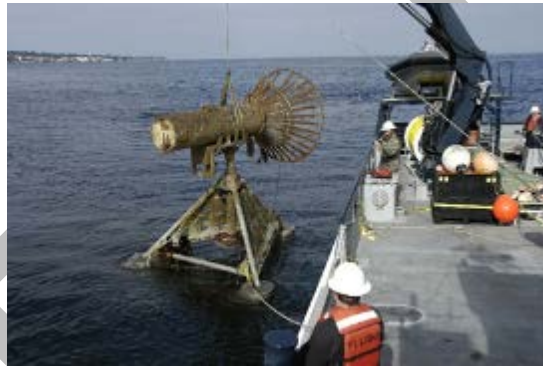
Figure 11. Docking station being recovered after deployment. Photo courtesy of MBARI (2017)
