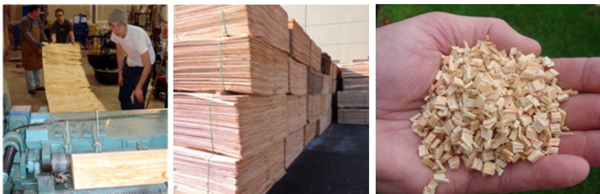
Figure 2–8. Veneering raw wood (a), stacked veneer sheets (b), and final Crumbles® product (c).
