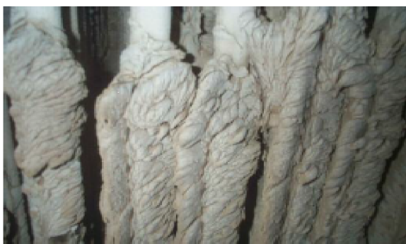
Figure 4–5 Secondary super heater fouling: potassium sulfate (left); potassium chloride (right).
