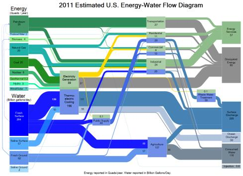
Figure 1. Hybrid Sankey Diagram of Interconnected U.S. Water and Energy Flows in 2011.
