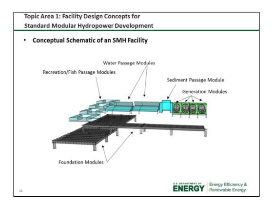
This figure illustrates a conceptual schematic of a SMH facility. This is just an example to show that the basic building blocks of the facility are individual modules that can scale across an individual site and across many sites.
