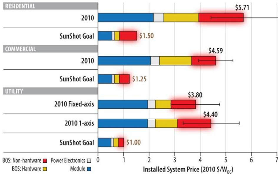
Fig. 3: Non-hardware balance of system (BOS) costs are represented by red bars. Prices are based on national average U.S. labor rates and exclude system operation, maintenance, and financing costs<sup>8</sup>.
