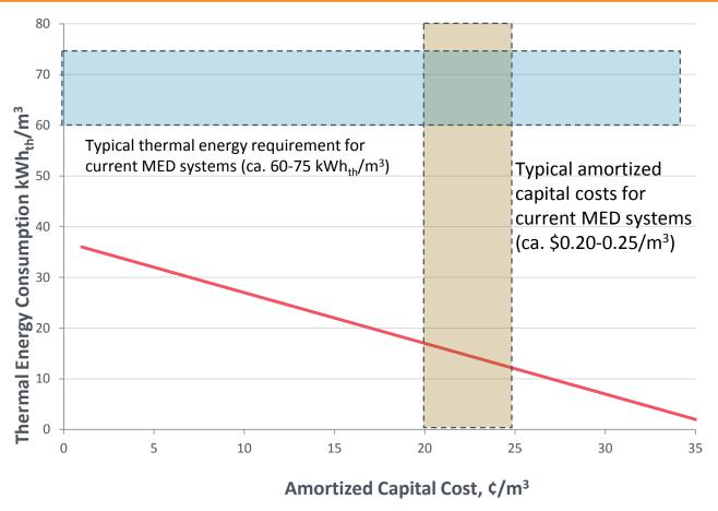
Justify how proposed innovations enable a thermal energy consumption and capital cost that fall on or below the red line (represents LCOW of \$0.50/m<sup>3</sup>)
