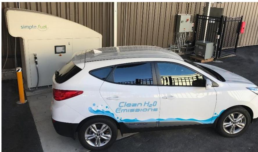
**Figure F1: The SimpleFuel H<sub>2</sub> dispensing appliance, illustrating the ease of refueling<sup>123</sup>**
