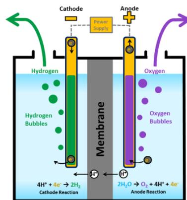
Figure C1: Electrolysis Schematic
