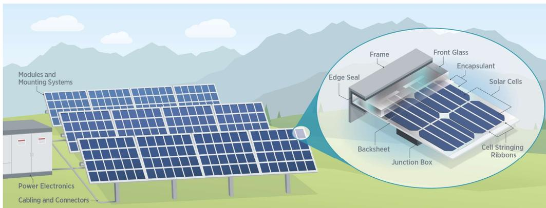
Figure 1. Components of a PV system. The inset shows the components inside a PV module.
